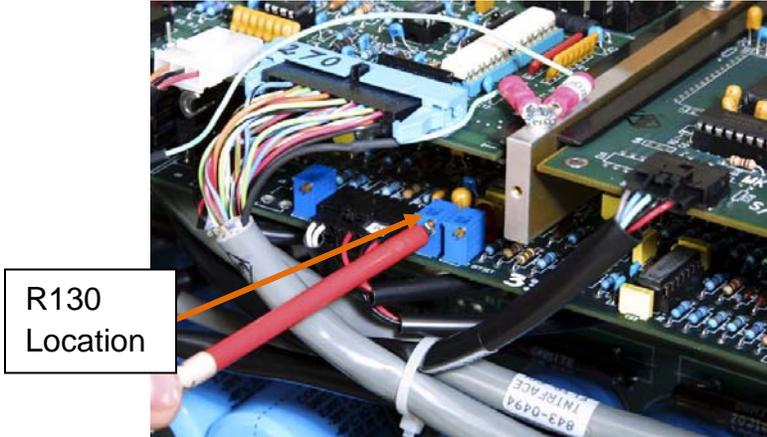
Fig. 4 – Trimpot R130 is used to adjust voltage at TP7
