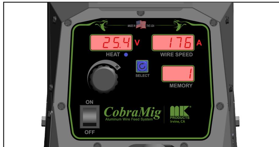
Note: Once arc is established during welding, actual welding Voltage and Amps will be live and displayed on the user interface. After welding, actual Volts and Amps will remain displayed for three seconds before resetting back to Reference Voltage and Wire Speed. See example above.
